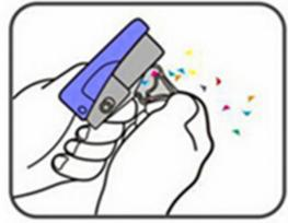
Uncover the other transparent side angle of the angle eater and pull out the chips.
