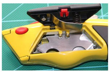
You can put 10 blades into the slot at most, and the common blades and hook blades can be put together.
