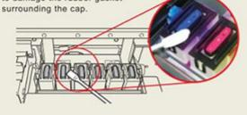
The accumulation of dirt around the cap gasket impairs the print head's seal to the cap. Over time, this problem can cause premature print head failure.
