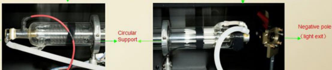
2. Electric wire connection—Connect the electric wires on both sides. Connect the red wire to the positive pole and the black wire to the negative pole. ;
