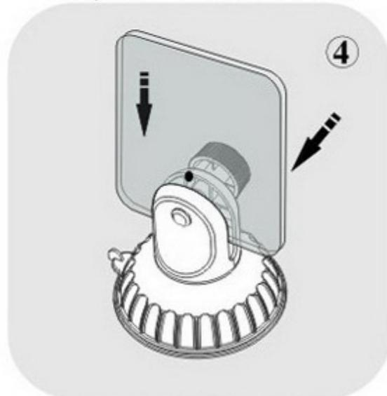
4、 Insert the drilled board into the channel on top, and fix it by screw.
