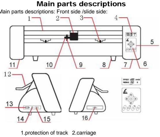
3.roller 4.LCD monitor 5.keyboard panel 6.LED lamp 7.right shell 8.machine's foot 9.knife holder 10.seat of knife holder 11.left shell 12.handel to control the roller 13.AC power port 14.safe fuse 15.power's switch 16.RS232 port
