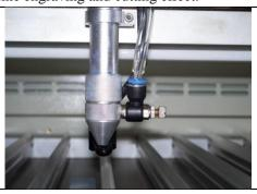
Laser head, with blowing device
