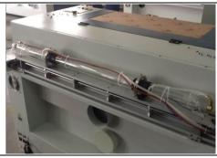
Equipped with 60W Chinese CO2 glass laser tube with fine engraving and cutting effect.
