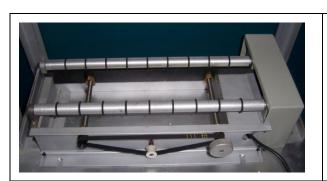
Cylinder Rotary Fixture: Used for engraving on the surface of column of  $\Phi 0$  - 150mm (0" - 5.9"), commonly used rotation clamp. +\$286
