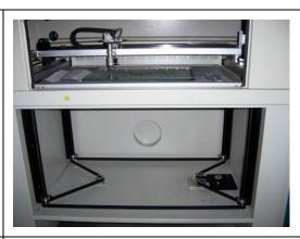
Equipped with electric up - down lift working table, its maximum lifting height can be up to 350mm (13.8").
