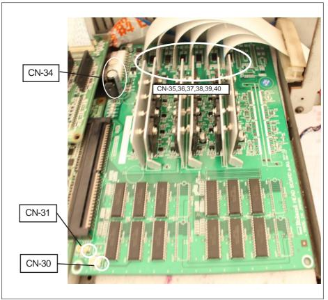
Disconnect the CABLEs from the HEAD BOARD.
