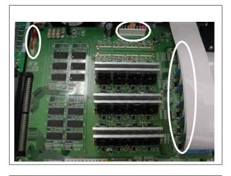
**2** Remove the screws shown in the figure to replace with the new Head Board.
