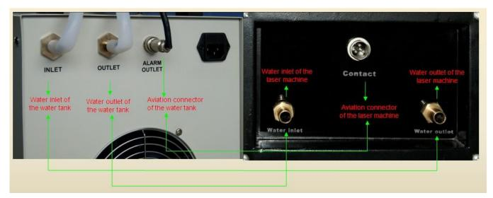
Industrial cooling machine's installation is very simple, the new machine for the first time using, you can install it as following steps.
