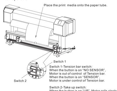
Switch 2-Take up switch: When the button is on "UP", Motor rolls clockwise. When the button is on "MIDDLE", Motor stops. When the button is on "DOWN", Motor rolls anti-clockwise.
