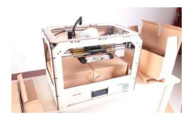
Under the build platform you'll find the filament -- either one or two rolls, depending on whether your Desktop 3D Printer has one or two extruders. It's easiest to remove the filament by first removing all of the remaining packing material.
