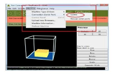
The software driver has not been installed if no port appears; let's install the driver. Click My Computer; right click select properties, then the basic system parameters appear. Then select Device Manager.
