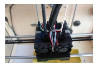
When the guide sleeve is disengaged, you can keep pulling the material from the guide sleeve behind the device until the thread passes through from the front.
