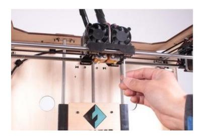
Next is the installation of the filament bracket. If you have two brackets, install one on each side; if you have only one, install it on the left hand side (when viewing the Desktop 3D Printer from the front).
