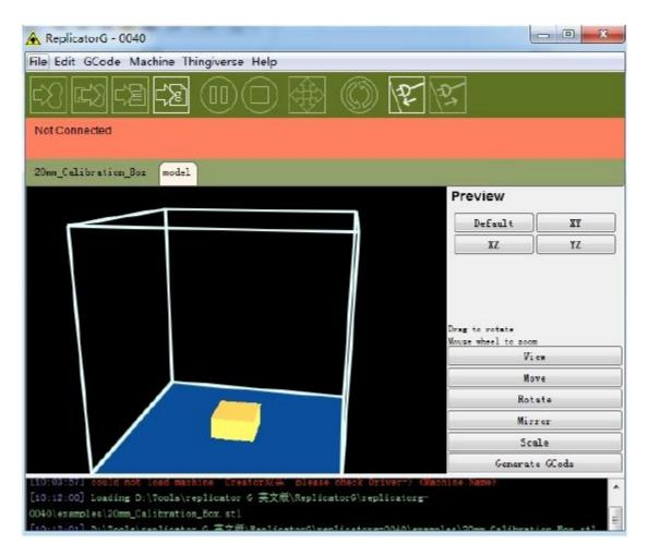
After the image is imported, there may be some problems, such as the diagram is unseen or the position is wrong. In that case, the following function keys can be used:
