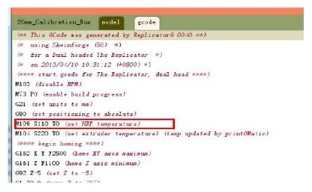
Then modify M109 S110 in red box TO (set HBP temperature) M109 S115 (set HBP temperature)
