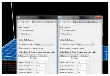
After G-code dialog boxes pop up, remove  $\sqrt{}$  before use base / support in the front, and then generate G-code one by one to.
