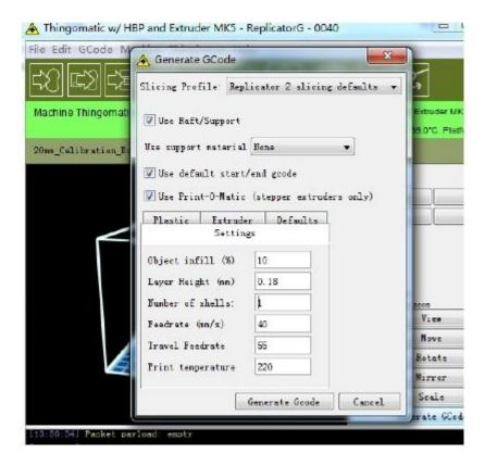
Filling ratio: the rate to fill the object -- 100% percent is solid.
