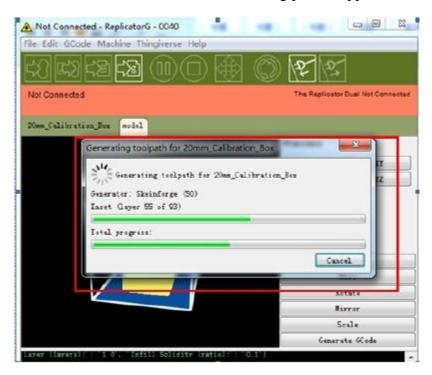
After G code is generated, the temperature of the bottom plate should be changed, please check the following picture for modification. First click G code in red box, and then change M109 S110 T1 to M109 S115.
