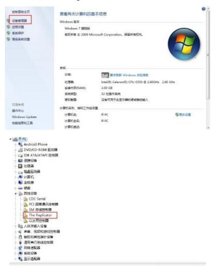
This software driver in the red box is not installed. Right click the Replicator, and
