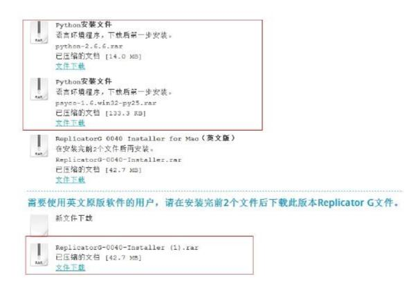
Download the 3 extracting packages in the red box and decompress them one by one. Then install the python installation file and python acceleration components. Then click replicatorg-0040 which is the decompressed file of replicator G.
