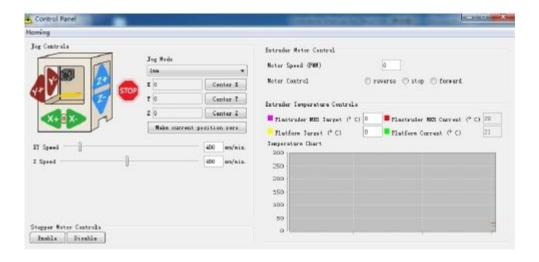
Input the target values. 220 degrees for the extruder (maximum 230 degrees); 115 degrees for the heating platform (maximum 120 degrees). After input, the platform will start to warm up. When the extruder temperature reaches 50 degrees, the cooling fan will activate and the current temperature value will display to the right, as shown below.
