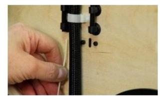
After the materials are inserted into the extruder, do not insert the guide wire tube into the extruder before the machine has started. There are two ways of feeding: one is to feed by using the LCD screen, the other is to feed using the control panel of the Print software.
