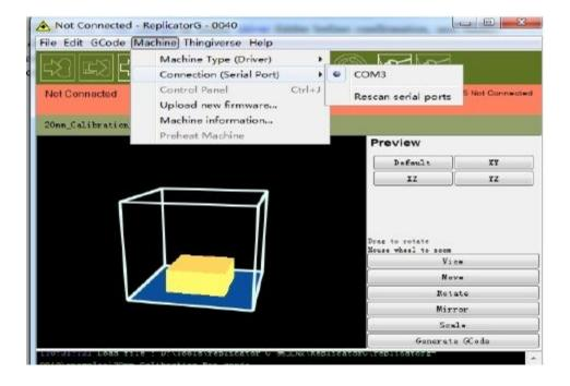
The port COM3 (this is the port for our test machine, it is different in each machine) appears. Click COM3.
