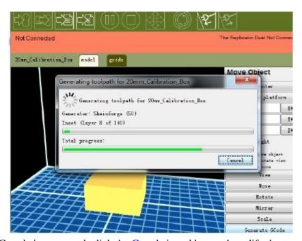
After G-code is generated, click the G-code in red box and modify the temperature of the bottom plate
