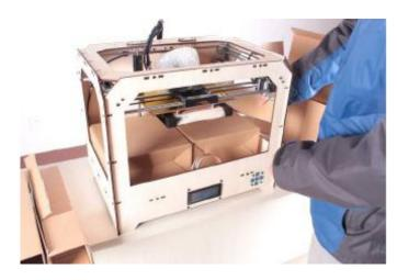
To do this, first take out the long box in the front, then the small box on the right, and finally the two wire trays.
