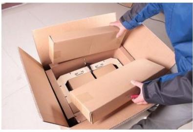
Now, you can see the top of the printer, as well as some cardboard boxes. The large box with the black wire is the **accessory box**, which includes **extruders** and other important components. Don't remove the accessory box or its contents, yet. Note: The black cable is not a handle! Do not use it to lift the Desktop 3D Printer.
