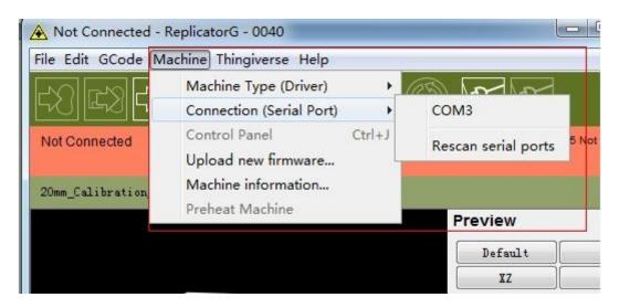
Choose the second option (Serial Port) on the menu, and we will find no port connected. Click rescan serial port, and the port will appear.
