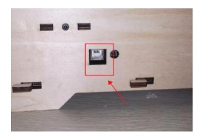
This is the USB port on the machine. After connecting the cable, open the software -- we are going to connect the computer and printer.
