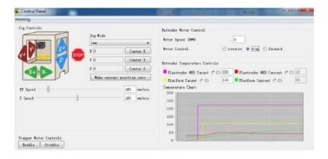
To heat the right extruder and feed material: click the right extruder in red box on the upper right corner of the control panel -- manually modify the temperature in the right
