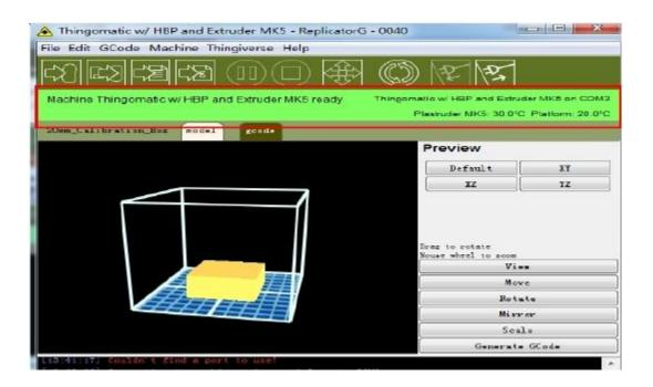
If red turns to green, the machine is connected with the computer. The next step is to heat the extruder and build platform.
