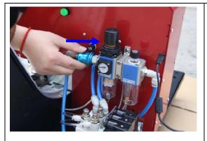
Turn on slide valve and connect pressure.
