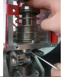
Press top die and loosen the set screw.
