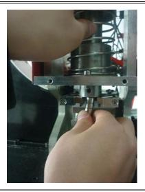
Remove the die and install a new one, then tighten screws.
