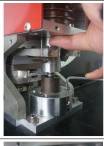
If the holes are not in the same side, loosen 4 screws, adjust the position of bottom die by moving the cylinder. Tighten 4 screws.
