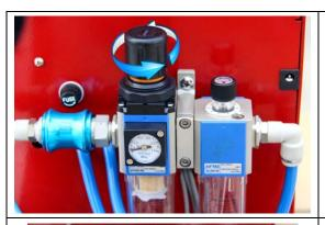
Lift up the knob and Rotate clockwise to increase the pressure.
