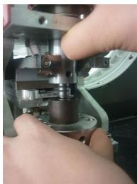
Depress top die slowly and make sure holes of screws are on the same side. If top die can insert into bottom die, top die will return to the right place. (Due to the gap between top die and bottom die is quite small, some slight frictions is normal and acceptable.)
