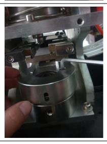
Flexible block must be tightened.
