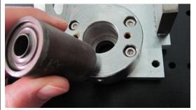
Loosen the set screw and remove the damaged die.
