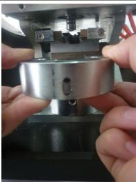
Press the flexible block to the bottom.
