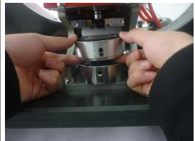
Press and remove the bottom die.
