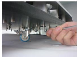
Loosen screws on the bottom. No need to loosen fully.
