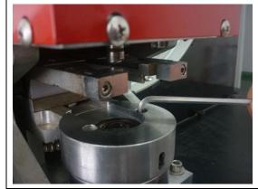
Loosen screws with M5 Allen wrench.
