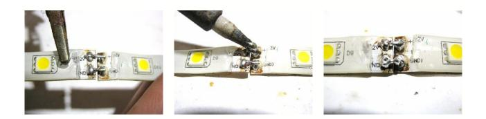
**Step #6:** Cover connection with hot melt glue and/or heat shrink tubing for extra protection. Be careful not to burn yourself!
