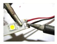
**Step #4:** Cut off the excess wires, with approximately 1/4" remaining. Pull off the sheaths from these wires, and pre tin them with solder.
