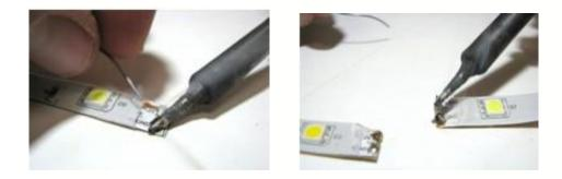
**Step #3:** Solder two pre-tinned wires onto the solder pads of the first strip. Try to stay consistent with red as (+) and black as (-). The wires should be long enough that you can hold on to them while soldering.
