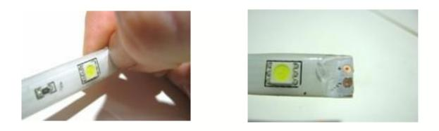
**Step #2:** With a hot, clean soldering iron, use Rosin-Cor solder to pre-tin the solder pads. It won't take long to heat the strip so be quick!
