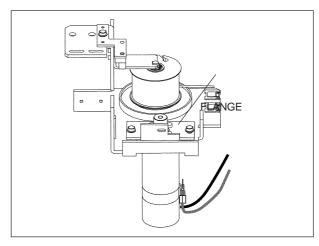
Fix the SPRING. Then, tighten up the 2 screws to fix the FLANGE with checking the gears mesh without backlash.
