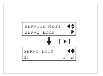
Press the [ENTER] key to excite the MOTOR.
