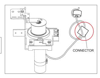
Connect the PANEL CABLE to the PANEL BOARD, and fix the PANEL COVER.
