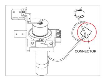
Remove the screws fixing the FLANGE and remove the MOTOR together with the FLANGE. Disconnect the 2 cables from the MOTOR then.
