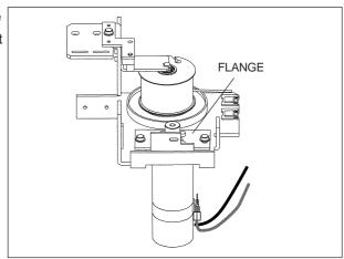
Remove the MOTOR from the FLANGE.
