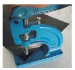
Step 5: Holding the handle at that level, align the material into position Step 6: Using both hands, completely depress the handle. to set the grommet.
