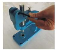
Step 1: Unscrew the nut and bolt at the top of the grommet machine.
