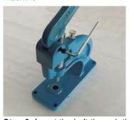
Step 3: Insert the bolt through the machine and handle, then tighten the bolt with the nut.
