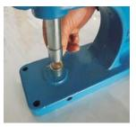
Step 1: Place the grommet on the bottom die.
