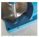
Step 3: Place the washer on the material.
