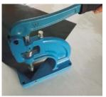
Step 4: Depress the handle lightly until the top die is touching the washer.
