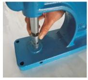
Step 5: Screw the smaller of the two piece Die to the location directly above the bigger Die.
