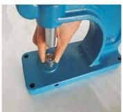
Step 4: Insert the bigger of the two piece Die into the hole of the bottom machine. Hold the Die in place by tightening the side screw.
