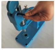
Step 2: Insert the handle with the larger side at the top of the machine
