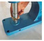
Step 2: Place the material on top of the bottom die.
