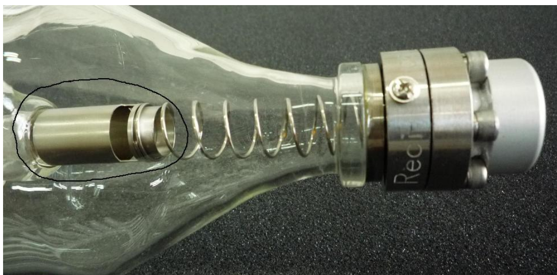
Negative electrode container
