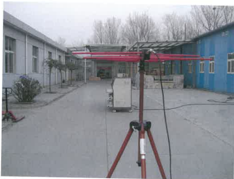
Photograph 4: Set-up for radio frequency (RF) emission, 300MHz-1000MHz, TTM-1700A
