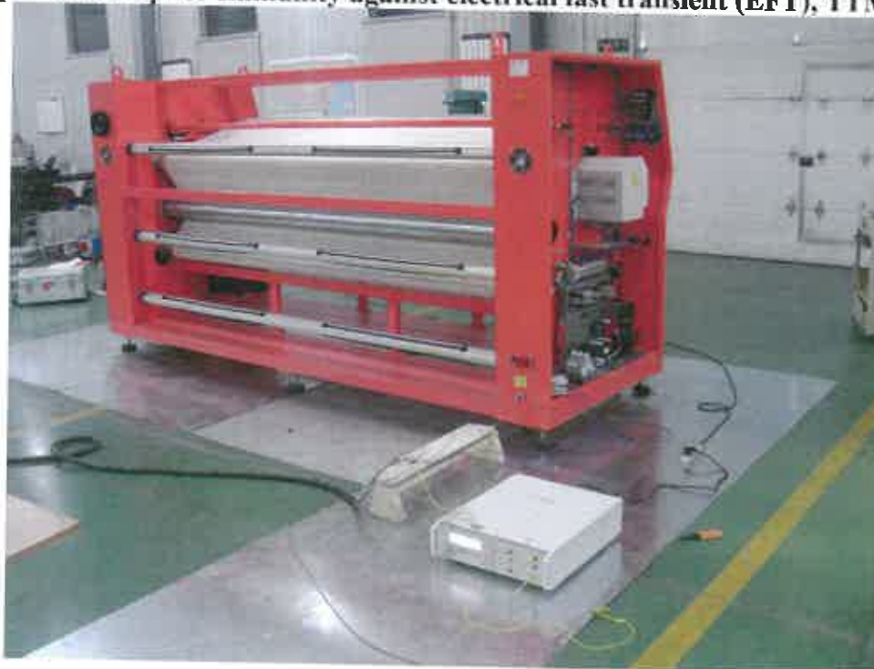
Photograph 14: Set-up for Immunity against electrical fast transient (EFT), TTM-2500
