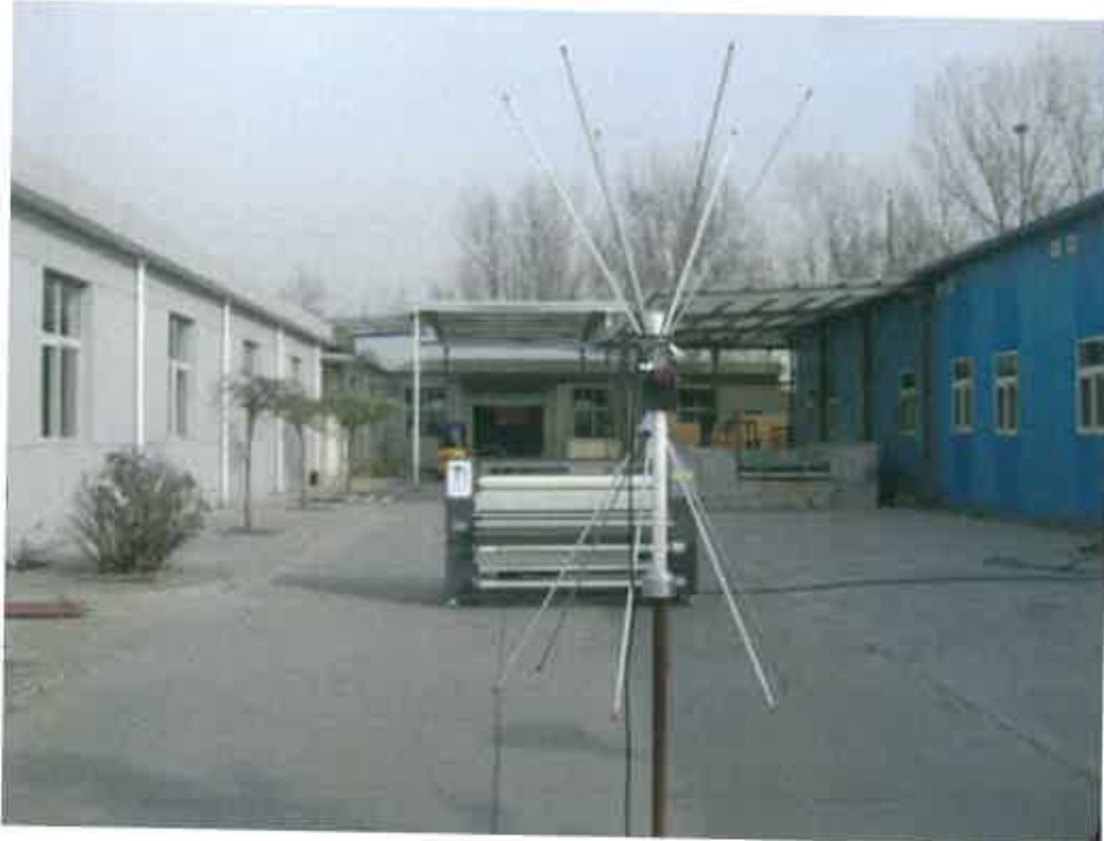
Photograph 3: Set-up for radio frequency (RF) emission, 30MHz-230MHz, TTM-1700A
