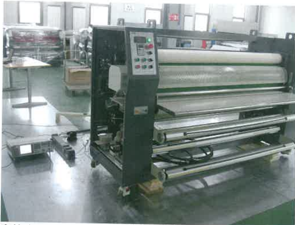
Photograph 10: Set-up for Immunity against radio-frequency continuous conducted, TTM-2500
