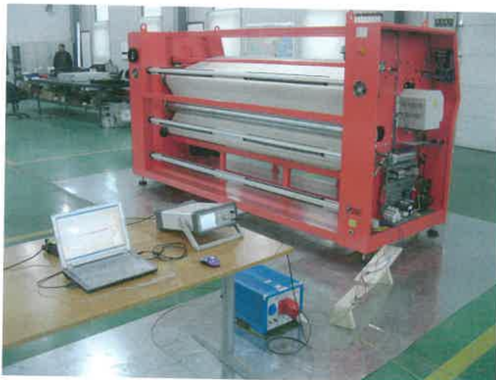
Photograph 2: Set-up for mains terminal disturbance voltage, TTM-2500
