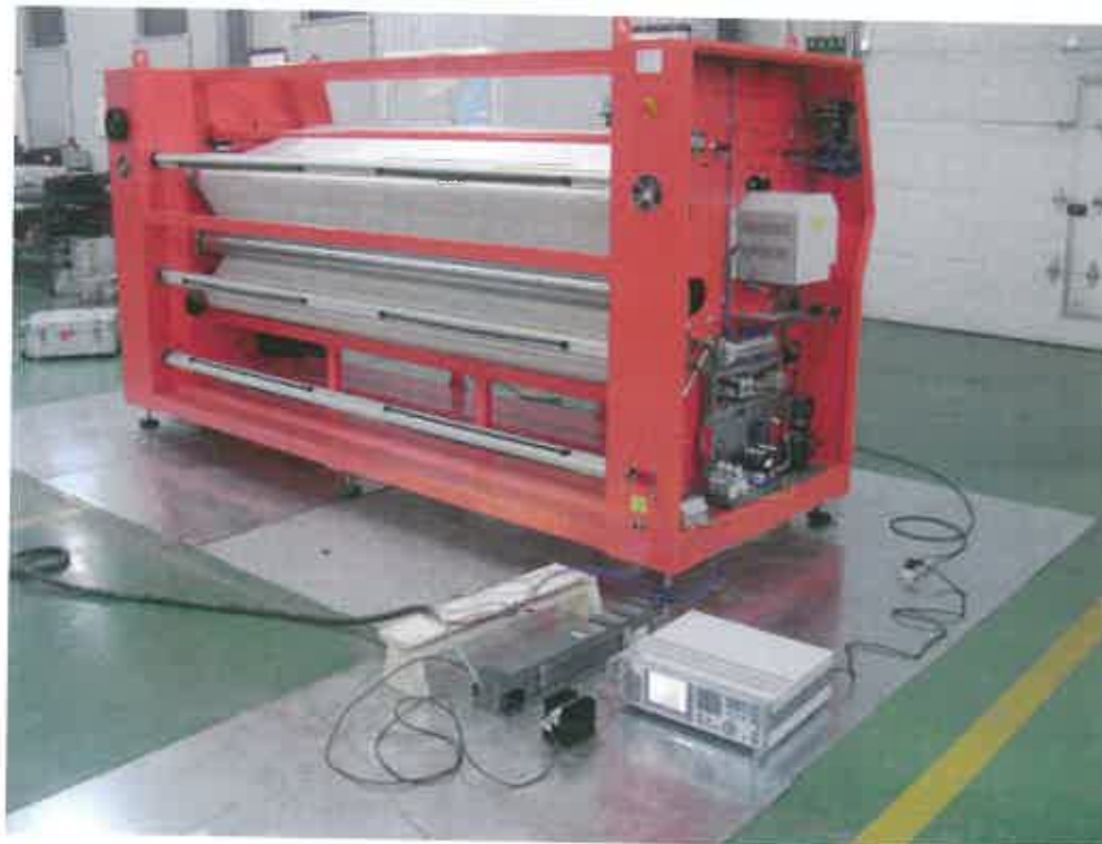
Photograph 10: Set-up for Immunity against radio-frequency continuous conducted, TTM-2500
