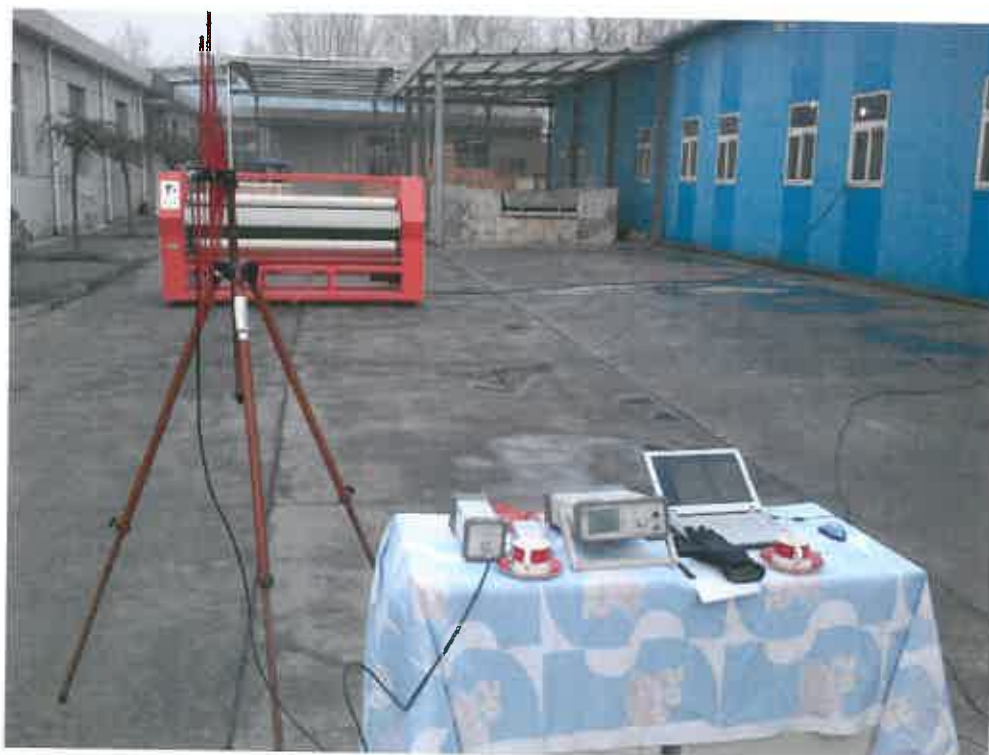
Photograph 6: Set-up for radio frequency (RF) emission, 300MHz-1000MHz, TTM-2500
