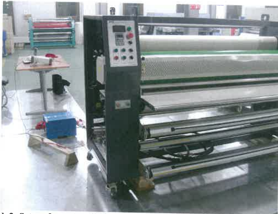
Photograph 2: Set-up for mains terminal disturbance voltage, TTM-2500
