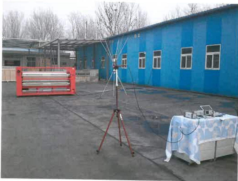
Photograph 5: Set-up for radio frequency (RF) emission, 30MHz-230MHz, TTM-2500
