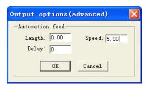
**Length**: after each processing, Z-Axis will feed a relevant distance for the feeding of the materials.
