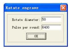
Pulse number in one spine: the pulse number needed for the spine axis spine once. Eg: driver is subdivided by 25 subdivisions, that is, 5000 pulse are needed in one spine. Reduction ratio of the spine table is 1:2, that is, input 5000\*2=10000 in this dialog box.
