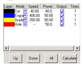
Process sequence is from the bottom of the list up. If you want to change the process sequence, simply check the line and click Up or Down will do.
