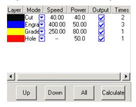
You can choose to output the layer or not in the "Output" column, ✓ is to output,
