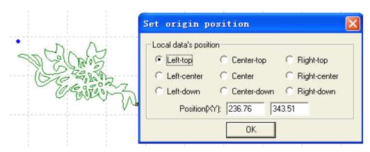
You can define the position of the left and right bottom as you need; move the mouse to any point to define the original point; input the position (x, y) to define the original point precisely.
