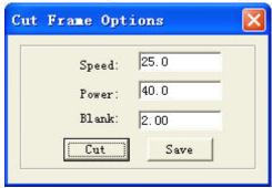
**Speed**: operating speed of the laser head in cutting. Different speed can be set according to the materials. It is better to define proper speed through testing.
