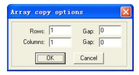
Input relevant parameters, identical figures with the number of the "lines×columns" will appear on the screen. The space between the figures will be determined by the "Backlash".
