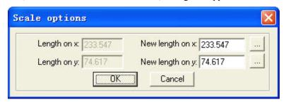
Input the needed length on the X, Y axis, and click "OK" to change the size of the figure. If you need to zoom in/out the figure with the same proportion, input the length on the X, Y axis and click will do.
