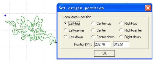
You may set left bottom, right bottom point of the processing data or move the mouse to any position; you may also input the origin (x, y) to set it precisely.
