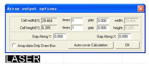
**Cell width (X)**: origin size of the processing data. **Cell height (Y)**: origin size of the processing data.
