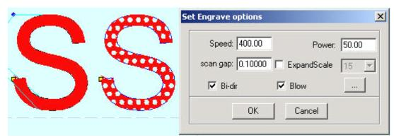
Figure on the right is the result with the "Fill circle" checked.
