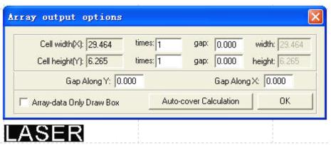
**Cell Width (Height) X/Y**: origin size of the processing data.
