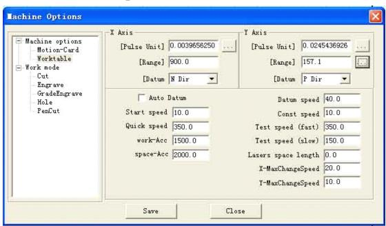
In Advanced Configuration, you can see after the range of the worktable on the Y-axis. Click it and dialog box appears as below:
