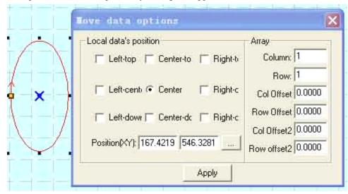
Input the corresponding (x,y) to make sure the coordinate of the data. See array setting in 4.5.3 Array Process Parameter.
