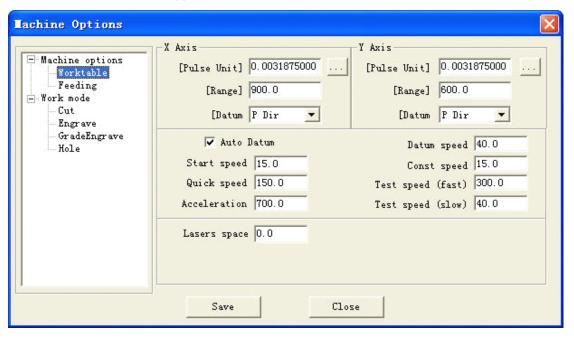
X-Axis is the horizontal axis, and Y-Axis is the vertical axis.
