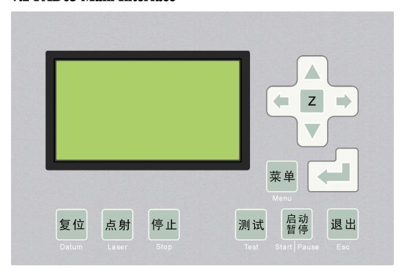
**Datum**: laser head move the original point of the machine slowly. It is mainly used to estimate cumulative error. You should make sure the application of datum switch and lead the switch signal to the controller.
