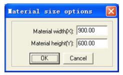
**Material Height**: length of the materials to process (default as the length of the worktable)
