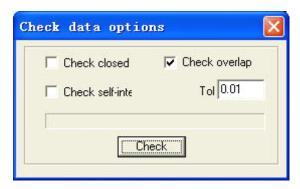
Check the "Aliasing Error": set the error of whether adjacent two nodes are taken as overlapped. If abnormal phenomenon appears in the processing (such as fail to engrave, cut twice), use the tool to check all the data. Abnormal data checked will be shown in the color of red. You can choose to delete or edit the node.
