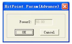
**Power2**: power of the second laser head. This function needs hardware support.
