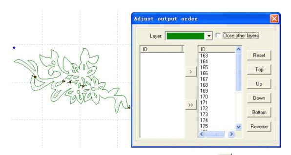
Click "Reset", select any figure, and then click "Space" or the button to move the ID number representing the figure to the list on the right. Order on the right list will be the process route in the cutting.
