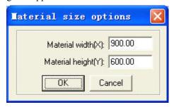
**Material Width**: length of the materials to process (default as the length of the worktable).
