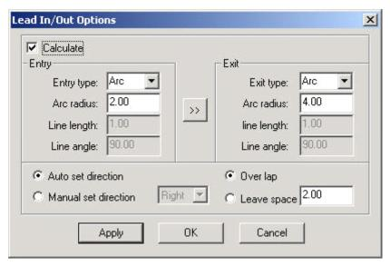
**Calculation**: this option can define the parameters of the lead-in/out line.
