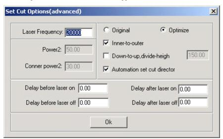
**Laser frequency**: control of the frequency of the laser's PWM signal in the process (mainly used to control the radio-frequency tube)
