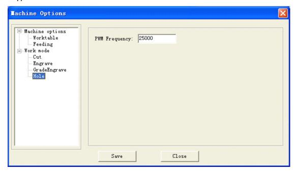
PWM frequency: It determines the PWM frequency of the laser power. It can adjusted between 200Hz-200KHz.
