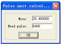
20.400000 in the picture above means the distance of the laser head moves every round of the motor is 20.400000 mm. 6400 is the pulse every round of the motor needs, and subdivision of the driver is 32.
