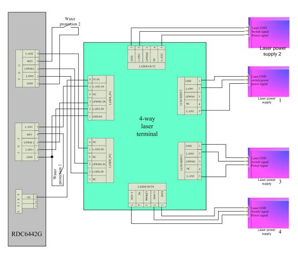
Notice: The power supply of laser expansion board are PIN 1& PIN 6 of LASER\_IN1, PIN1 is GND, PIN6 is 5V, so you should connect PIN6 to one 5V terminal of four controller driver interface, due to the strong power supply capacity of 5V terminal of X/Y/Z/U driver interface.
