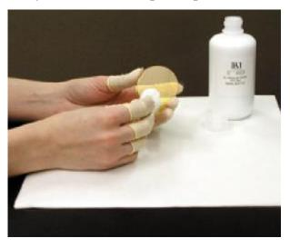
For severely contaminated and dirty optics, an optical polishing compound may need to be used to remove the absorbing contamination film from the optic.
