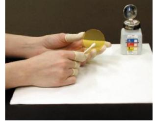
cotton swab in the optic's center and clean outwards in a spiral motion toward the optic's edges.]
