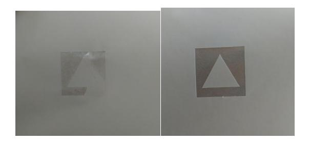
When you put the material and knife installed, open the machine, press the test button, the machine will automatically cut a square and triangle,
