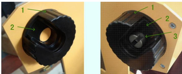
1.Plastic lock cover 2.Plastic lock 3.Liner slot
