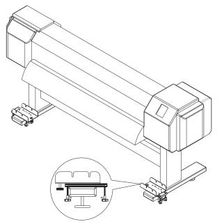
Install linking slabs to printer stand, pay attention to installation direction.
