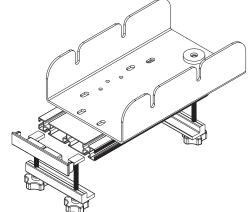
Open plastic cover and slip the fasteners into aluminum bar, then install the cover.
