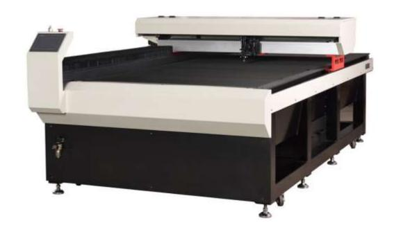
The G-1325 CO2 laser cutting machine offers high precision and large format cutting solution for acrylics, wood, cardboard and other materials.
