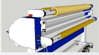
Put on the paper tube for the finishing media collecting rod.
