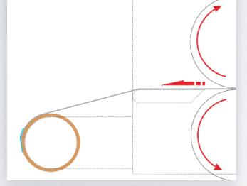
Tape the laminated media to the collecting rod when the length of output is enough.
