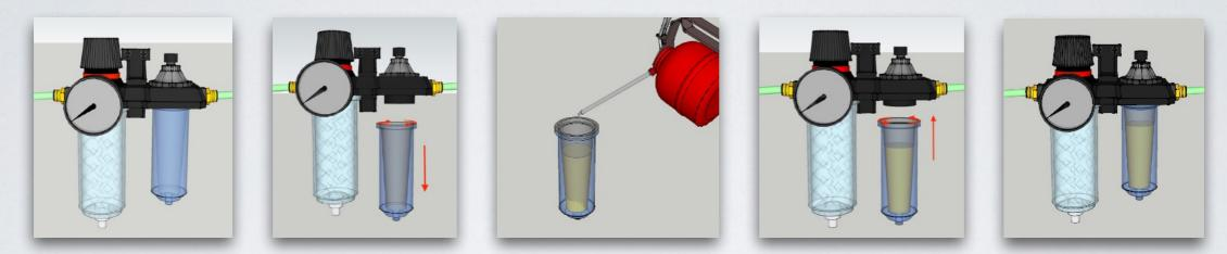
(Regular adding lubrication oil could improve the stability of the air cylinder and lengthen its life.)
