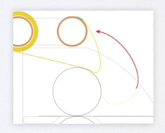
When laminating the film onto the media, please keep pulling the back paper up to the back paper loading rod. Then tape it to the collecting tube.
