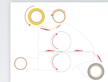
Then step on the feet pedal to make the roller rotating in forward to output laminated media.
