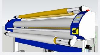
Put on the media for the media loading rod, also put on paper tube for the back paper collecting rod.
