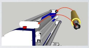
Put the film roll back, into the bracket slot.
