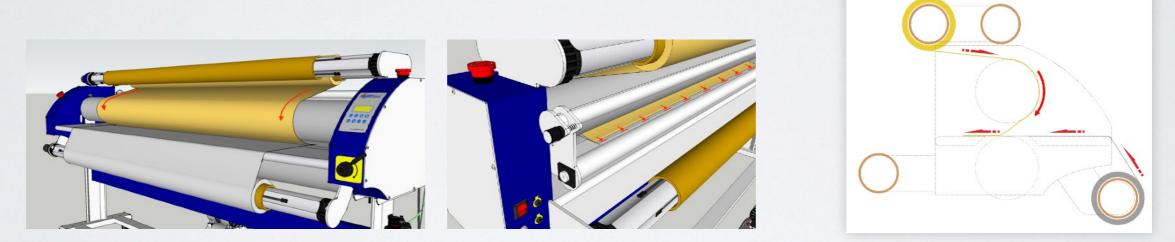
Pull the end of the film roll down, through the bottom of up-roller, make sure the end of film roll align to the end of the media.
