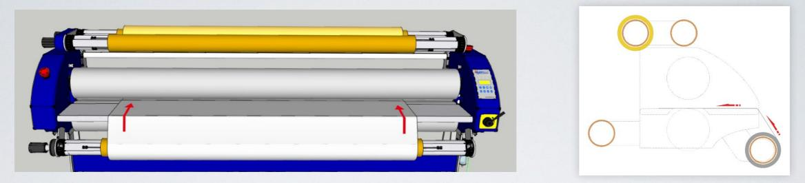
Pull the end of media up to the front platform, then flatten it, ensure the media end cover and over the rollers around 15cm.
