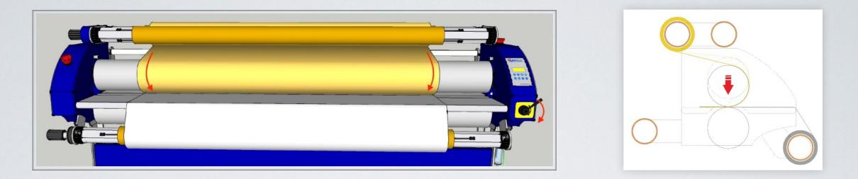
Then press the middle of media by hand while twist the valve handle in clockwise direction, to fall down the up-roller, which will fix the media and the film, ensure there is no any relative movement between them.
