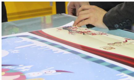
9. Slide the guide beam slightly and manually to finish the whole lamination.
