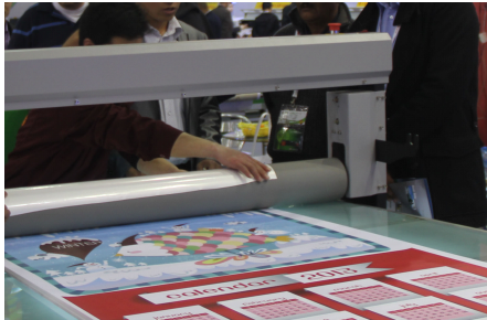
9. Slide the guide beam slightly and manually to finish the whole lamination.
