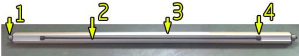
1 Bearing 2 Rubber strip 3 Aluminum shaft 4 Scale mark
