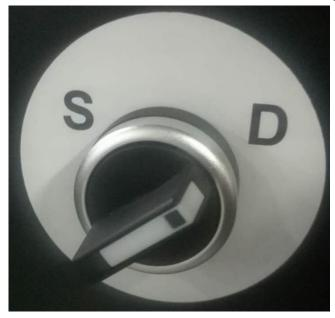
When the user selects dual-jet mode, press the start button, and the spray car will start to spray from the origin and move to the position of set length, and then automatically return to the origin. The nozzle is always in the spray state during the whole process
