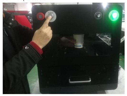
Description: when the cleaning button is pressed, the liquid pump will start to work. The liquid pump will take out the treatment liquid in the liquid bucket, and then spray out evenly through the fan nozzle
