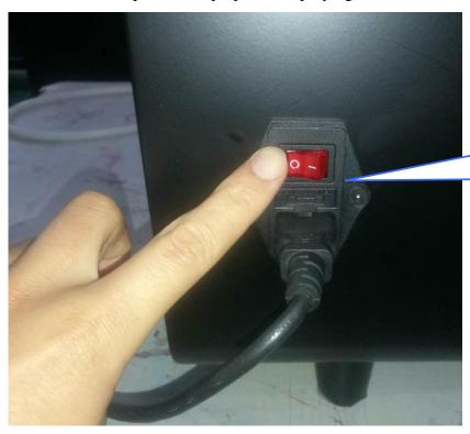
Insert the power cord and turn on the power switch
