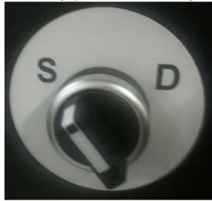
When users want a smaller amount of spray, they can choose the single spray mode. In the single spray mode, press the start button and the sprinkler cart will stop spraying after it moves from the origin to the setting length position.
