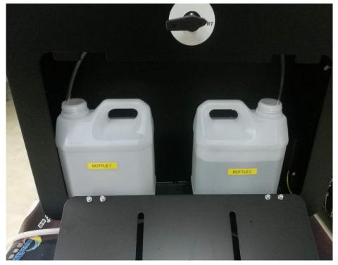
Clear water (pure water) in bottle 1 Bottle 2 contains the treatment solution
