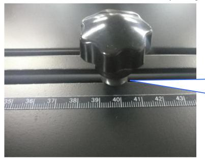
The position of the hand screw on the ruler is the length of the spray on the T-shirt
