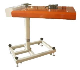
The flash dryer is an important piece of equipment in the screen printing process, especially in multi-color printing. you can dry the ink quickly to print next color by flash dryer. it's specially combined with t shirt carousel screen printing machine.
