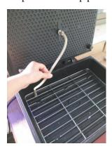
Move → vacuum pump is ok, check sealing strip, vacuum pipe and vacuum plate etc to see if there some place leak air.
