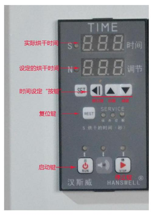
Reset key: When the machine runs about 300 hours, the module alarm, three LED lights, the need to promptly clean up the electric box and filter, press the RSET key to return to normal.
