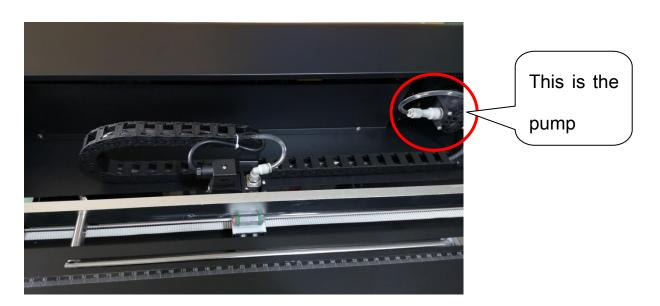
Please check the tube connect to the pump is empty or not
