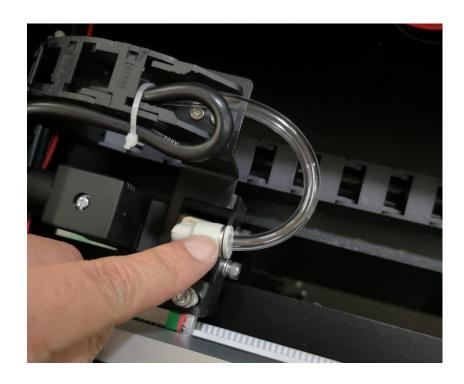
This is the quick connector, Pull off the tube from the quick connector
