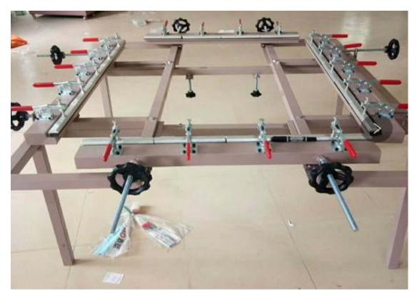
4. Finally, install the girder on the four sides and install the handwheel
