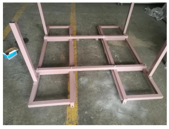
2. Connect the two iron stands with two square pipes
