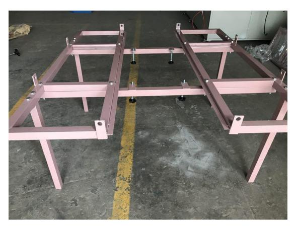
3. Turn the iron frame over and install four rubber screws
