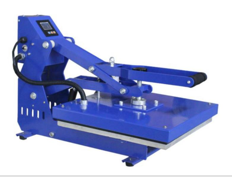
The press is equipped with a manual override, a digital display, and a sound signal at the end of work.
