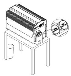
2.2.3 Plug in, press the power switch, adjust the three-way switch, turn to spray. Press the working switch some times to check the spray status, ensure spray completely(This step is to confirm there is no air in tube, ensure the coating liquid are full with tubes). Pull out the platen, put the t-shirt smoothly, close the platen and press the working switch. Take down the t-shirt after spraying, repeat.
