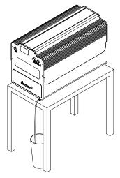
2.2.2 Pull out the containers, according to the marks to add the coating liquid and cleaning liquid(normal pure water).
