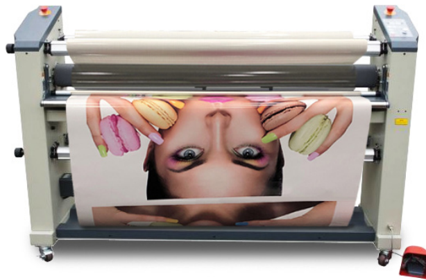
Working table with ruler, which makes the feed table is more stable and the laminating effective is better.
