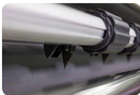
Rear table with cutting unit
