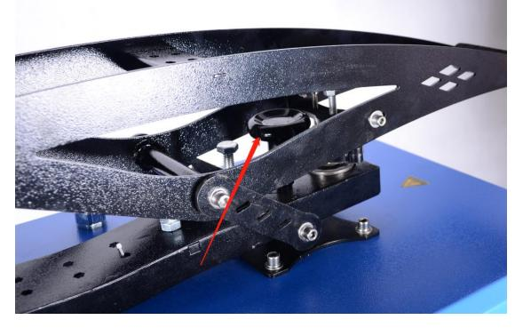
**Time**: If the transfer time arrives, but the buzzer does not ring or stop ring, then you need to check the micro-switches point of
