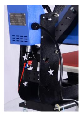
**Temperature**: when the time arrives ,the pointer of the thermostat is at the place of zero .(Temperature up to 180  $^{\circ}$ C requires about 15 minutes.) ; if heating plate does not heat, please check the circuit.
