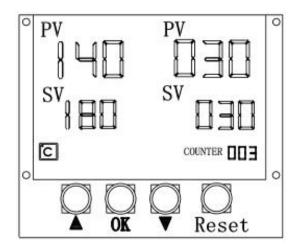
2. Press the "OK" button will shows the degrees Celsius "C". You could use the Up or Down button to switch between degrees Celsius and degrees Fahrenheit.
