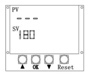
4. Press "OK" button to enter TIME setting. When the TIME indicator SV(right) blinks, use Up/Down button to set the required time. (Time adjustable range: 0-999S)
