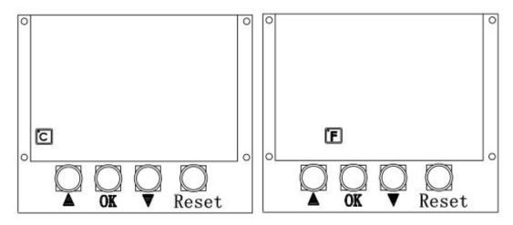
3. Press "OK" button to enter TEMPERATURE setting. When the TEMP indicator SV(left) blinks, use Up/Down button to set the required temperature. (Temperature adjustable range: 0-225 o C/0-437 o F)
