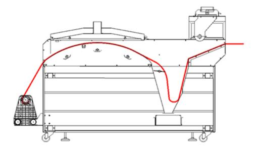
**2.1** Lead the media into powder box, though outside powder bar, and then cross the space between up dryer and platform dryer, wind the media to the paper tube of
