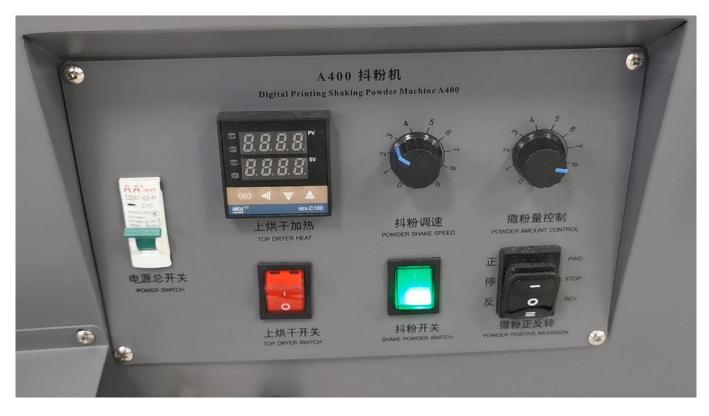
**1.1** Confirm that the external power supply of the equipment is connected with AC110V, 50 / 60Hz.
