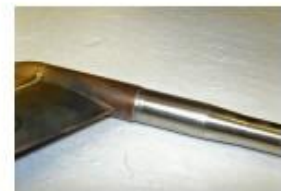
Probe for a CRJ jet made of beryllium copper and nickel
