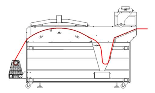
**2.1** Lead the media into powder box, though outside powder bar, and then cross the space between up dryer and platform dryer, wind the media to the paper tube of
