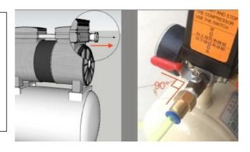
Ensure the Red button on the top of the air compressor staying pressed Then we plug in the power for Air compressor
