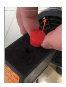
Pull up the Red button to start the Air compressor to compress the air. 1 ~2 minutes later, the Air compressor will stop automatically when the pressure coming to around 0.8Mpa.
