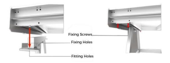
Screw the Oil-water Separator onto the stand frame, just like below showing:
