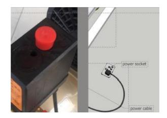
Pull up the Red button to start the Air compressor to compress the air. 1 ~2 minutes later, the Air compressor will stop automatically when the pressure coming to around 0.8Mpa.
