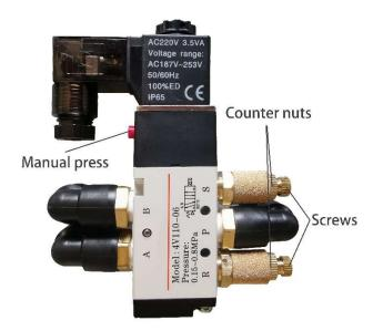
• On the side of the solenoid valve there are two silver/golden screws which restricting the air flow speed of the cylinder.
