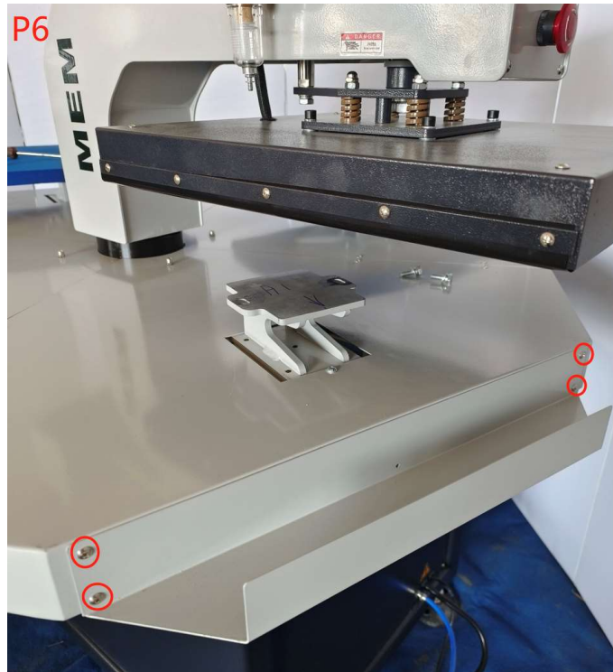
P6: Install the fabric tray (it is designed for long fabric press job, which can prevent the fabric from fall off, this part might not needed for regular t-shirt press)
