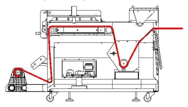
**2.1** Lead the media into powder box, though outside powder bar, and then cross the space between up dryer and platform dryer, wind the media to the paper tube of the take up winder, the winding operation complete.
