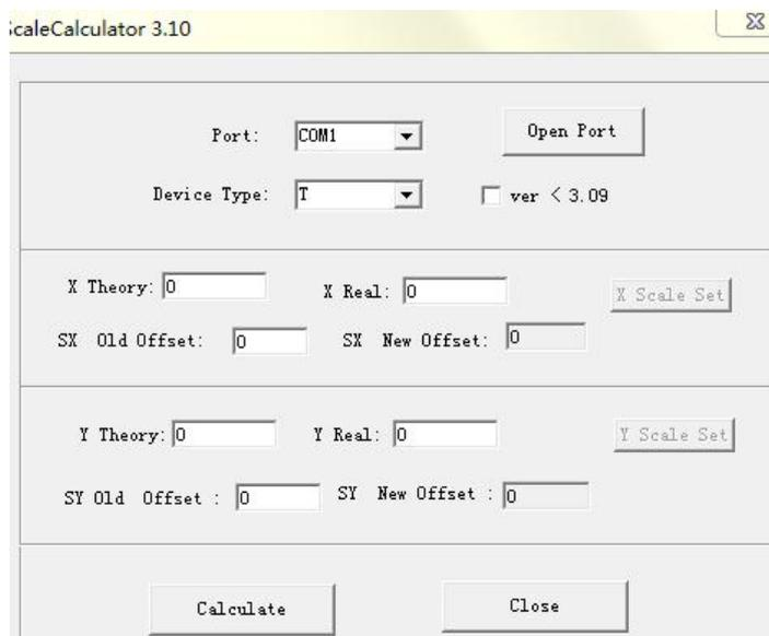
It needs us to cut a 400\*400mm pattern. And then measure the actual cutting size. Use the scale calculator . Put X theory / Y theory value 400mm, X real / Y real is real cut value. Device type: T. Click Calculate.
