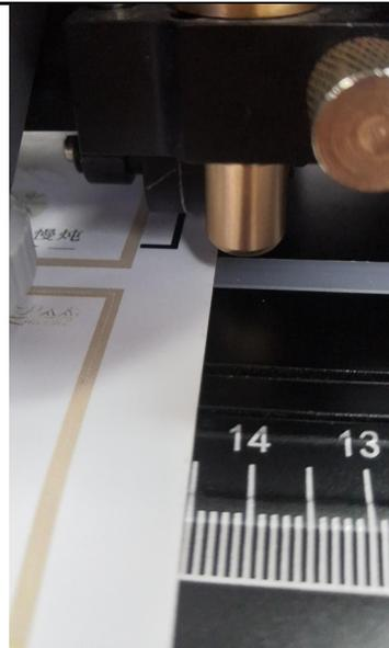
The golden knife holder is placed on the edge of the material
