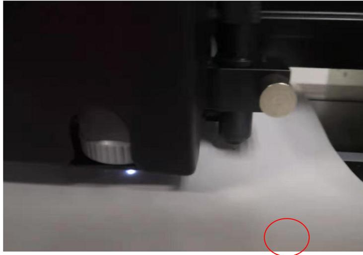
Change the knife holder to a drawing pen and press down on the drawing pen to leave a small dot on the material. Then click the calibration page, after it becomes DX set DY set, the white light of the scanning head will be on. Then press the arrow keys to move the sports car to make the white light coincide with the black origin, and then press the OK key on the screen to save the parameters.
