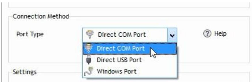
When you connect the machine and computer by using USB cable, choose the “Port type” “Direct COM Port”.
