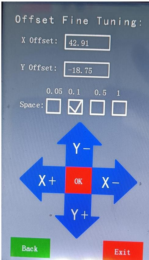
Left and right deflection, adjust the X-axis offset;
