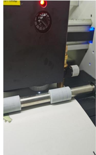
The white light is on the blank material, the red light is on, the white light is on the black position, and the red light is off.
