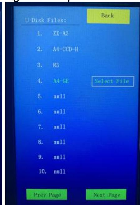
Operation method: Insert the U disk into the machine port, click "U Disk" to enter the second page, and then click "..." to enter the U disk file menu. Select the corresponding file name and click "Choose File" at the back. The machine starts working.
