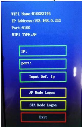
Mobile app connection method: open the mobile app, click the wifi button, the name of the current nearby WiFi will be displayed, find the WiFi name kaola007 displayed on the machine, connect (no password); then click on the "network settings" on the mobile app, enter, enter The IP address displayed on the machine, that is, the port number, select "AP" for the working model, and click "Keep Settings".
