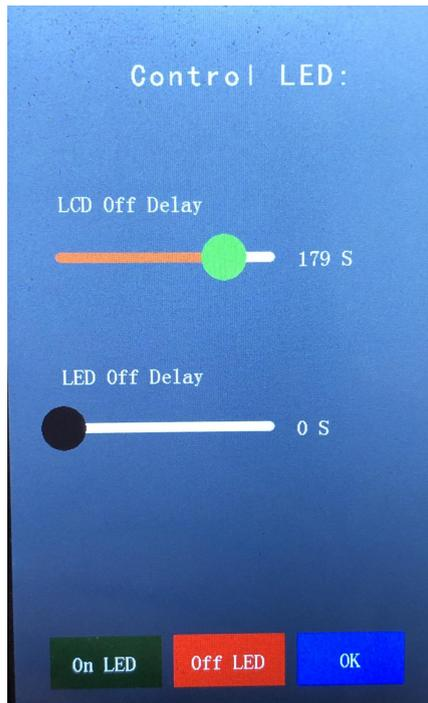
If your machine with LED lights, When click “Control LED”, it goes to the interface. You can set the LED lights on time manually.
