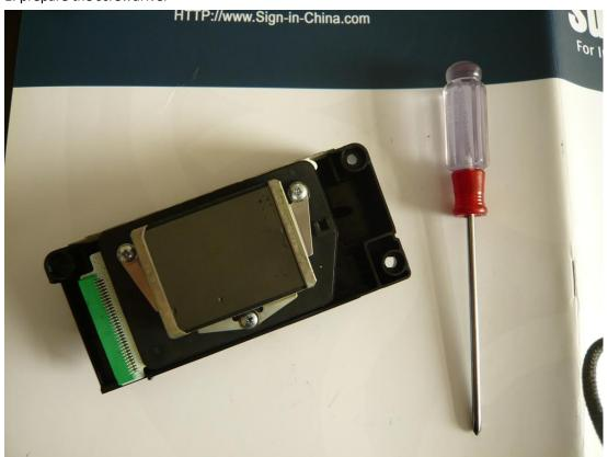
2. Screw down the 3 screw on the printhead
