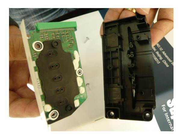
6. align the printhead with the new adapter and install
