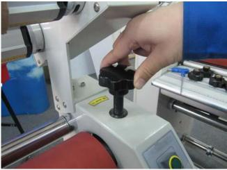
Step 4. Power "OFF" the machine, set direction to F, rotate speed setting at very low value like 2. Insert prints and align both sides refer to laminating film, you can look the front working table mark ruler also, make sure the prints is straight and smooth enough, and then press Pedal switch to run machine. Then press button "ON" and release pedal switch running at auto mode. You can adjust tension by rotating brake knob to get good laminating result.
