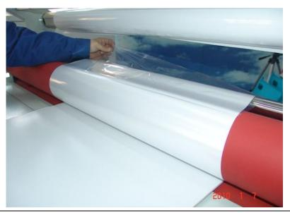
Step 5. Manully peel liner, and then press Pedal switch to run mounting. Step 6. Mouting finish.
