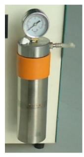
**Fourthly,** Switch on the power, the indicator light turns bright, the fan begins running; gas can be felt out of the outlet (within 1 minute), the pressure gage indicates 0.01-0.05mpa. If you seal it with a finger, the gas pressure will go up until over 0.1mpa and the ammeter indicates zero; move out the finger, the gas pressure will go down and the ammeter indicates well. All these mean that the machine is normal for working.
