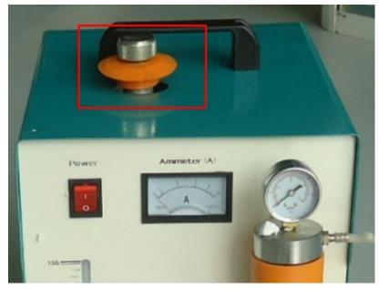
**Thirdly,** unscrew the filter bottle cover, put the alcohol into filter bottle up to one - third place, and screw the cover.
